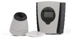
Infrared Beam Detector with automatic adjustment by an infrared sender and receiver unit including a reflection prism. The Fireray 5000 requires 1 prism for the range of 8-50 m and 4 prism for the range of 50 to 100 m
